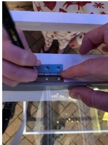
Attached the cover with two hinges.
