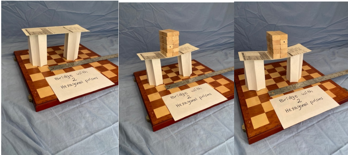
The bridge made from two hexagonal prism was able to hold 10 small blocks (300gr) and on the second test it held 12 blocks (360g)
