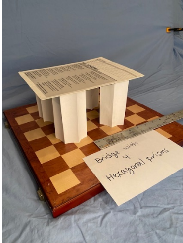
The Bridge made out of four hexagonal prism columns was able to hold 26 small blocks (416g)
