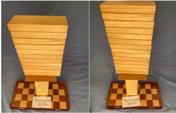
The Rectangular Prism was able to hold 11 blocks (1,430 g) and on our second test 14 blocks (1,820 g)
