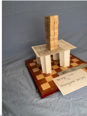
The Bridge made out of four hexagonal prism columns was able to hold 26 small blocks (416g)
