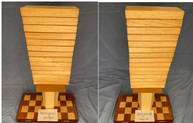
The Pentagonal Prism was able to hold 14 blocks (1,820 g) and on our second test, 15 blocks (1,950 g)
