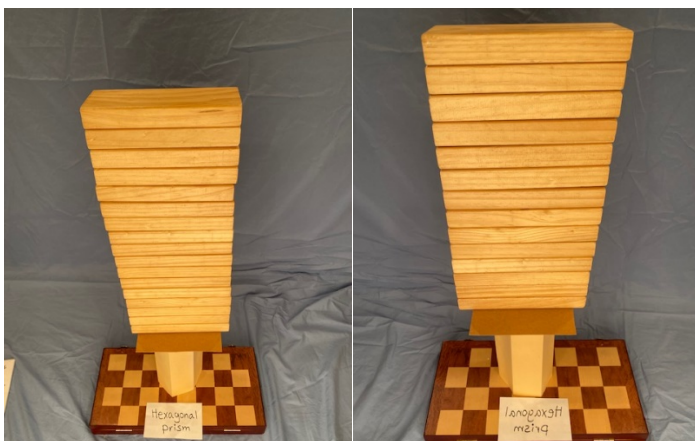
The Hexagonal Prism was able to hold 14 blocks (1,820 g) and on the second test, it was able to hold 17 blocks (2,210 g)
