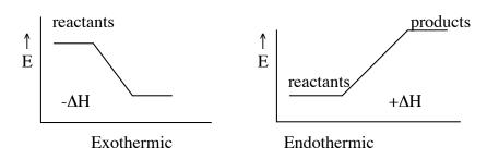
Activation Energy- the energy need to start an exothermic chemical reaction. For an Exothermic reaction- add heat/spark/
