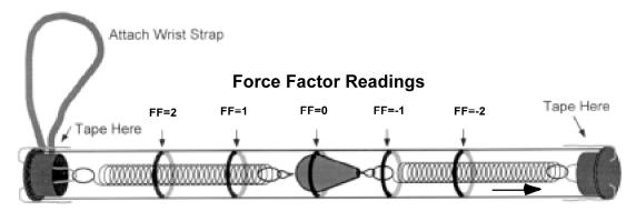
**Above:** The two-spring Force Factor meter can measure positive and negative Force Factors. **Below, at Left:** A single-spring homemade Force Factor meter. Oriented vertically, the current reading is a Force Factor of 1.0, meaning that the upward normal force on the meter equals the gravitational force on the meter.
