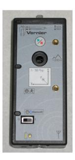
**Above Center and Above Right:** Vernier's 3-axis "accelerometer" and their Wireless Dynamics Sensor System are devices that would be secured in a data vest worn by someone riding the ride. Because these sensors are fixed in orientation relative to the rider, the coordinate axes for measurement are named
