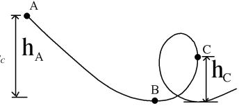
Thus by measuring the speed of the train at point A, and the heights  $\mathbf{h}_{A}$  and  $\mathbf{h}_{C}$ , the speed of the train at point C can be calculated.
