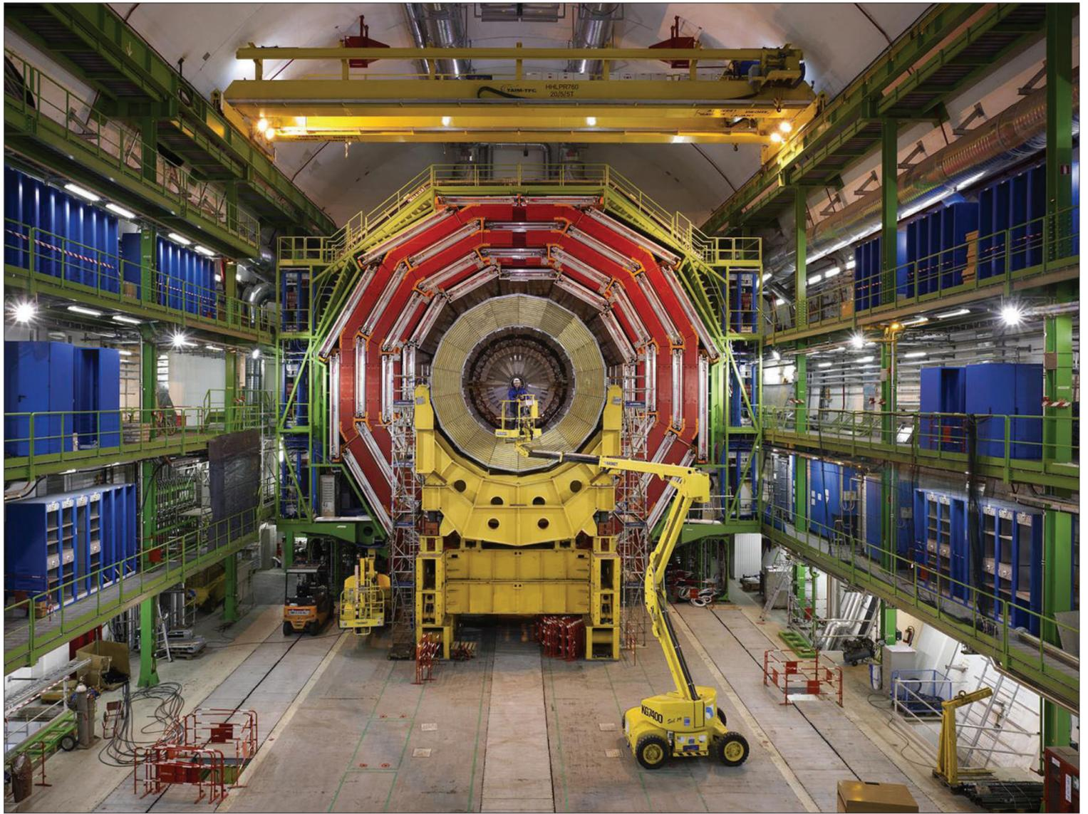
A 13,000-ton particle detector is installed in the Large Hadron Collider, the world's largest atom-smasher, in Geneva, Switzerland.
